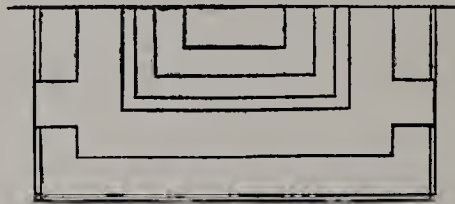
FIG. 75.—Plan of stages for lean-to house. Scale, \frac{1}{8} inch = 1 foot.
